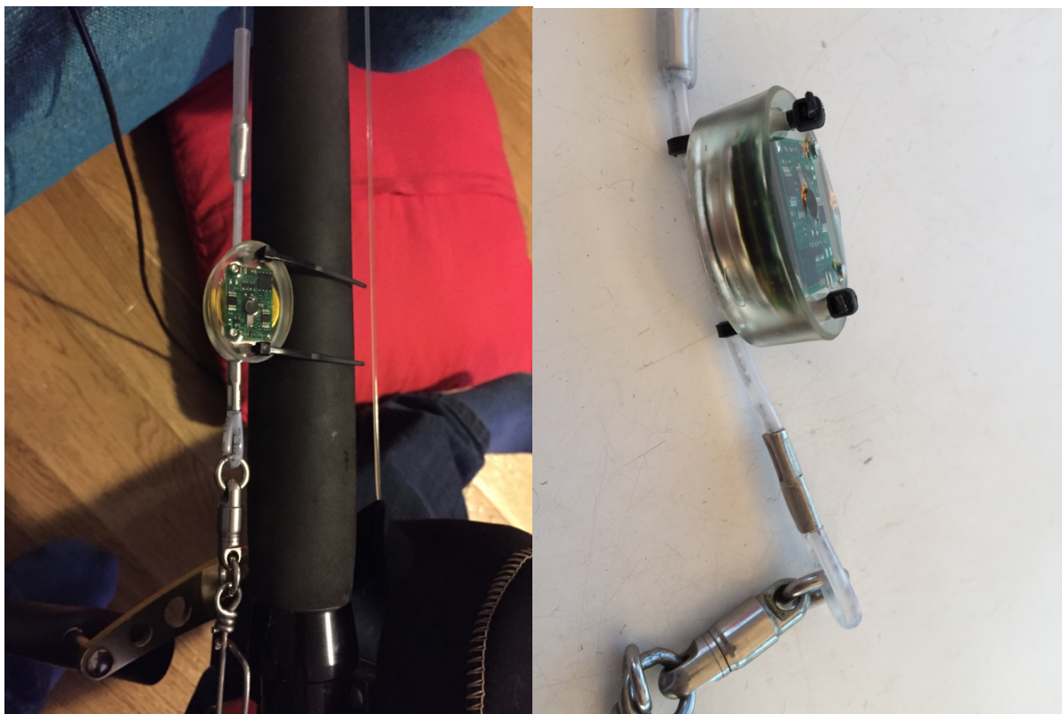
Figure 3. Accelerometer attached to the terminal tackle of the research fishing gear.
